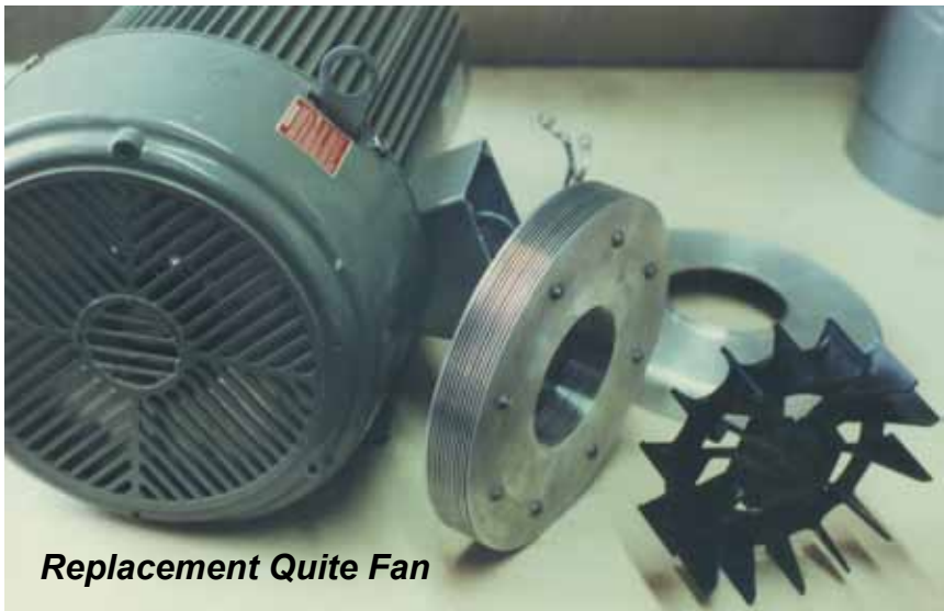
Conventional Noisy Bladed AC Motor Cooling Fan
