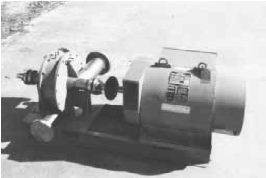
General Ener-Tech 200 KW Salt Brine Geothermal Turbine
