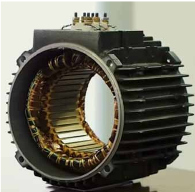
Induction Motor Stator Rotor Removed
